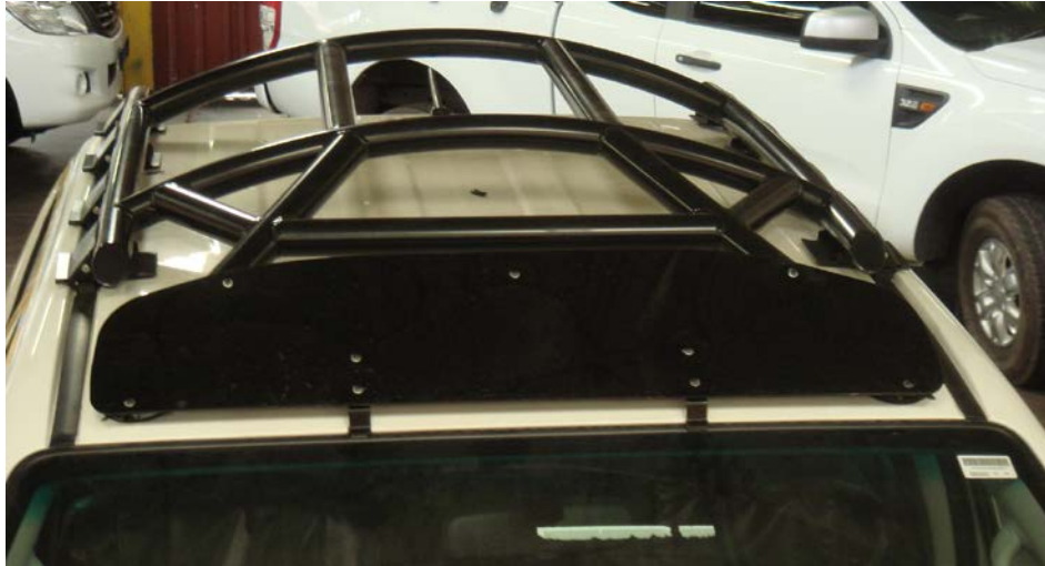
Figure 1. Patented aftermarket HALO™ ROPS fitted to a Toyota Hilux Dual Cab Truck
